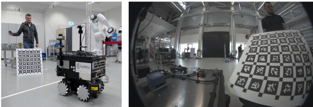
Figure 1: Our use-case is the calibration of pinhole and fisheye cameras in robotics applications using dedicated calibration targets (e. g. checkerboard patterns, April tag grids).
